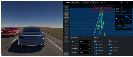
Fig. 3: Illustration of LGSVL simulator (left) and Baidu Apollo ADS (right).
