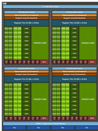
Illustrating 1 SM in NVIDIA Ampere GPU [1]
